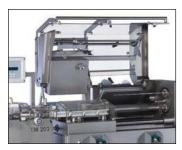
Switching from collagen casings to natural casings couldn't be easier. Simply raise the casing loading magazine for easy operator access to the twin stuffing horns.
